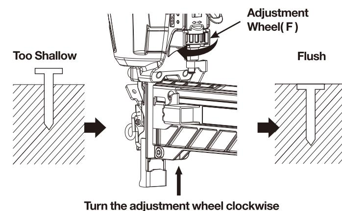
**CAUTION:** It is advisable to test the depth on a scrap workpiece to determine the required depth for the application.
