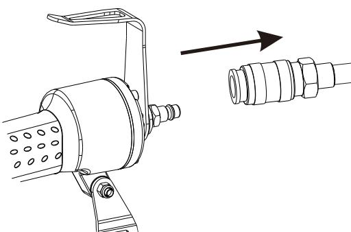
2. Turn the tool so the air inlet is facing up. Place 2 - 3 drops of pneumatic fastening tool oil into air inlet. Do not use detergent oils, oil additives, or air-tool oils as these lubricants will cause accelerated wear to the seals and bumpers in the tool, resulting in poor tool performance and frequent tool maintenance.
